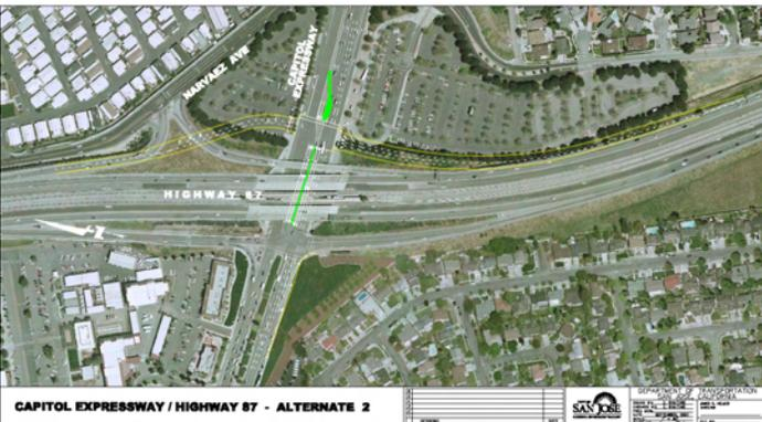
**Alternative 2:** Replace the existing on/off ramps. Build new direct northbound 87-to-Capitol off-ramp and northbound 87
