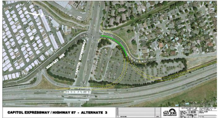
**Alternative 3:** A loop ramp configuration adding alternatives to the existing 87 onramp on Narvaez. For eastbound Capital traffic, the Route 87 on-ramp loop would be a free right turn near existing westbound Narvaez. Northbound 87 traffic could exit directly to Capitol via loops to Narvaez on both sides of the interchange. Estimated cost = \$25M.
